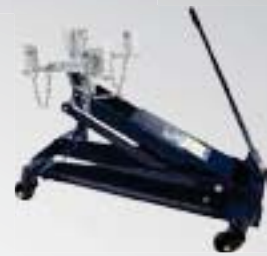
1 TON Transmission Jack Saddle Forward Tilt 68 Degree Saddle Reverse Tilt 15 Degree Rated Capacity: 2000 Lbs. Lifting Range: 8-1/4" to 30-5/8"
