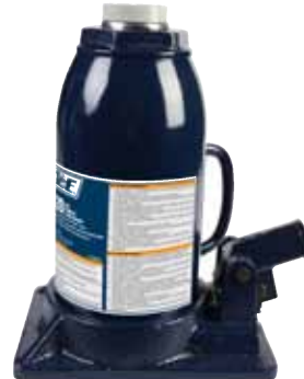
20 Ton SKU 451486 TCE92007 119 99 • Rated Capacity: 40,000 Lbs • Stroke: 7-15/32" • Adjustable Screw Extension: 3-3/8" • Lifting Range: 10-7/8" to 18-3/8"
